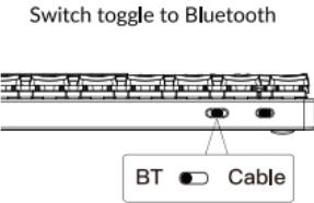
Press fn1 + Q (for 4 seconds) and pair with device named Keychron K7
